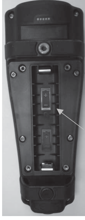
Figure 1. Pro Plus with battery cover removed. Notice battery symbols indicating polarities.
