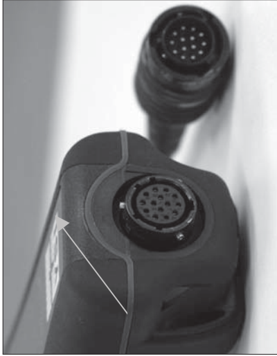
Figure 5. Note the keyed connector. The cable and instrument connectors can only be mated once the keys are properly aligned.
